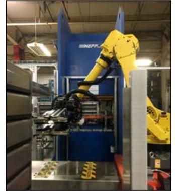
Figure 3. Hydraulic press for forming aluminum parts in a robotic manufacturing cell.
