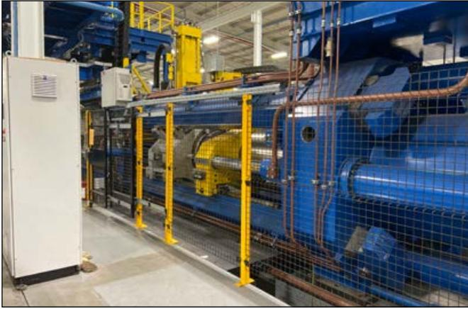
Figure 1. The new extrusion press is capable of processing profiles up to 25 ft in length.
