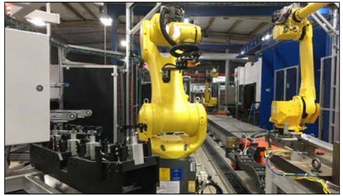
Figure 4. New robotic cell for high-volume manufacturing of aluminum rails for the automotive industry.
