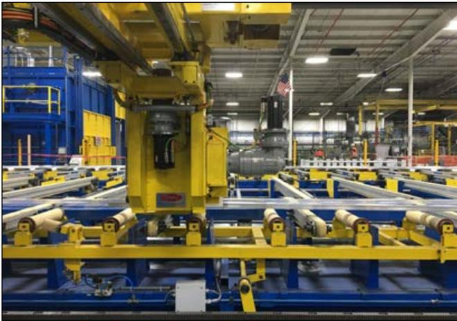
Figure 2. Electric double puller with flying hot saw.
